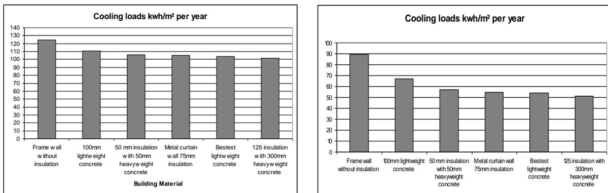
Fig. 5: effects of changing U-value and building materials on the cooling loads
