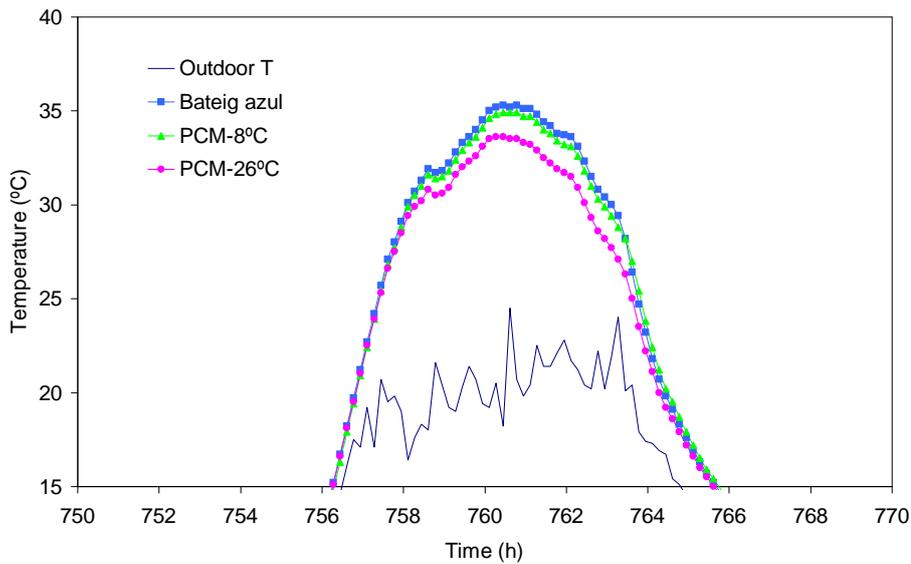
Figure 6. Temperature inside adiabatic boxes with one side of Bateig azul with and without PCMs. Effect of different melting temperature of PCMs during summer.
