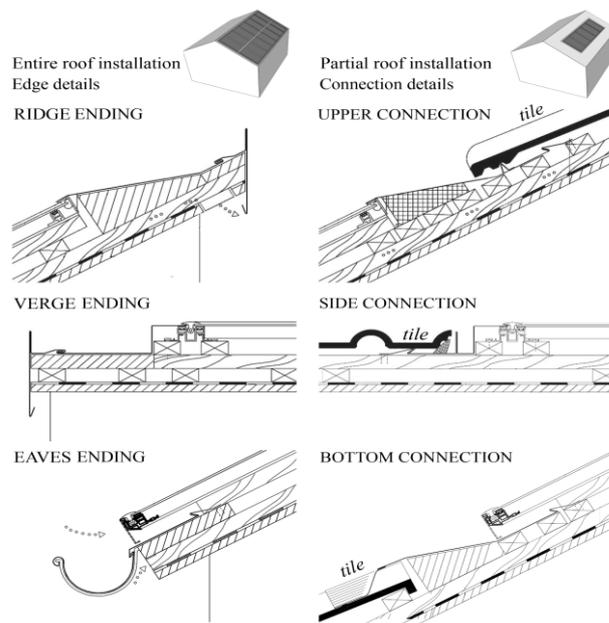
Figure 3: Details of entire and partial PV integrated roofs (Solar World AG, 2008)
