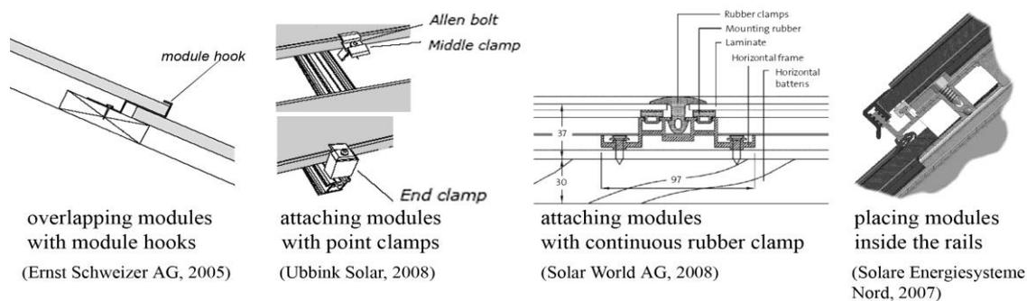
Figure 4: Module fixings
