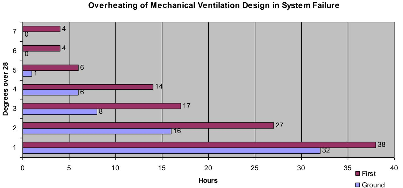
Figure 6: Overheating of final design stage of the Mechanical Ventilation design strategy: number of hours at each degree over 28°C to a maximum of 35°C
