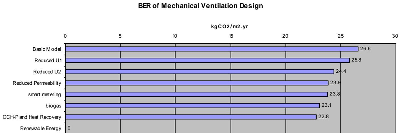
Figure 5: Building Emissions Rates of design stages of the Mechanical Ventilation design strategy
