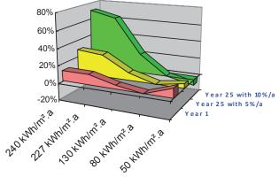
Figure 3: Additional occupancy cost in social housing compared to low energy retrofit (base 100).
